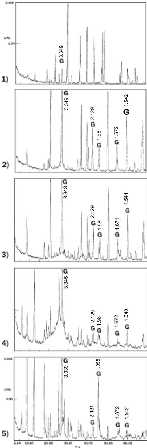
Figure 3. X-ray diffractograms of graphitization material from Tepeköy (1), Tatköy (2, 3) and Meydanköy(4,5).
